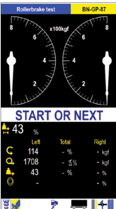
inner left wheel locked during brake test
